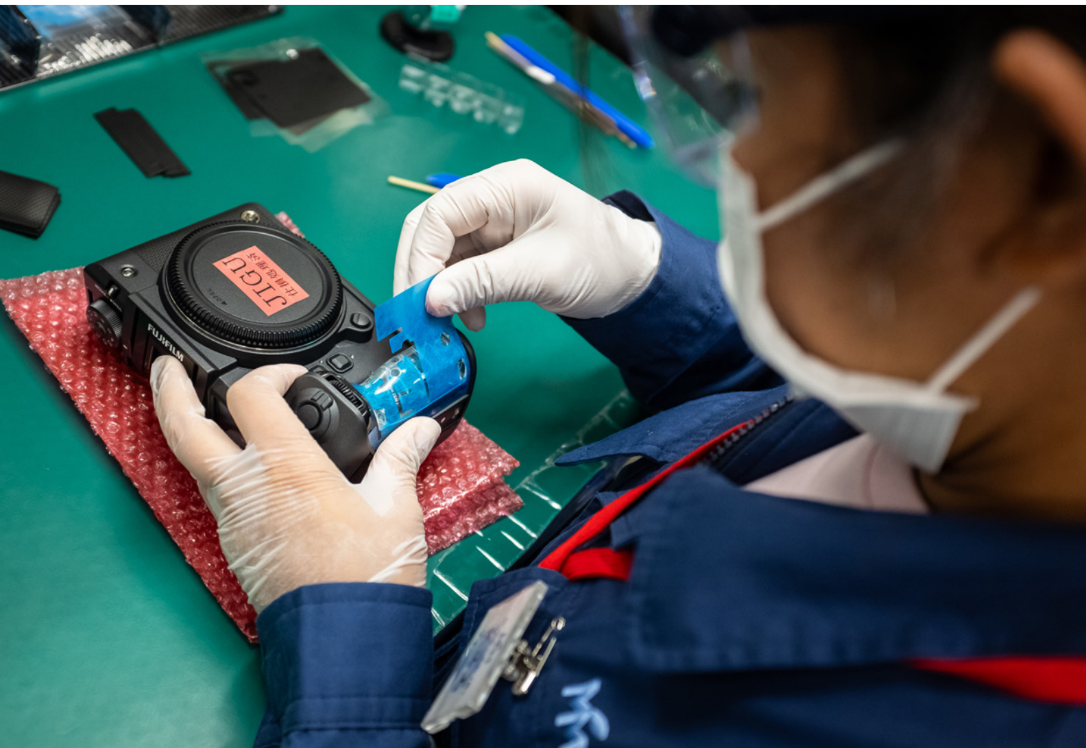
Above you can see the technician putting the rubber grip on the grip side of a GFX100 II. She did a remarkable job and in one-fifth the time it took me.
