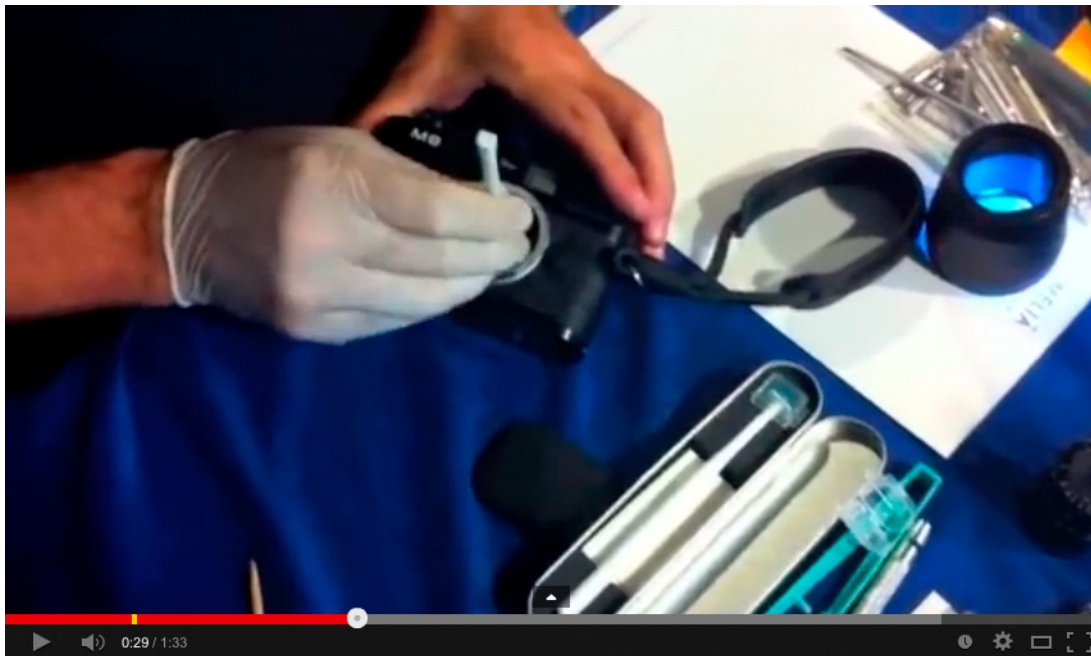
Above is a screenshot of a video showing a Leica tech cleaning a Leica M9 sensor with the Sensor gel Stick. So, just in case you wanted proof that the big camera companies use this tool to clean sensors when you send a camera back to them, here it is. Click on the screenshot above to view this video on YouTube.
