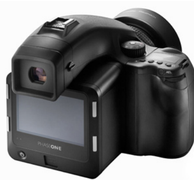
The 36-megapixel Nikon D800 (top) and the Phase One 645DF camera with the 80-megapixel IQ180 digital medium format back (bottom) mounted on the back of it.
