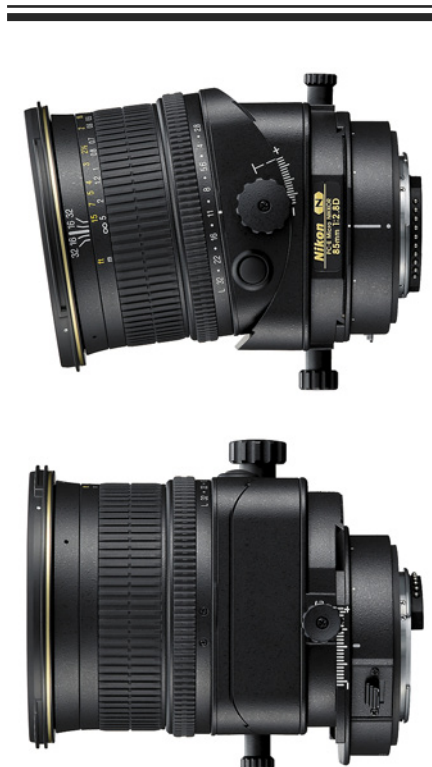
Above is the 85mm f/2.8D PC-E Micro Nikkor in the tilt mode (top) and the shift mode (bottom). The focusing ring is at the far end of the lens with the aperture ring just behind it. Note that there are four main knobs to control the lens, one for tilting, one for shifting and two for locking tilt/shift movements. The knobs are arranged with one on each of the four sides of the tilt/shift adjustment.
