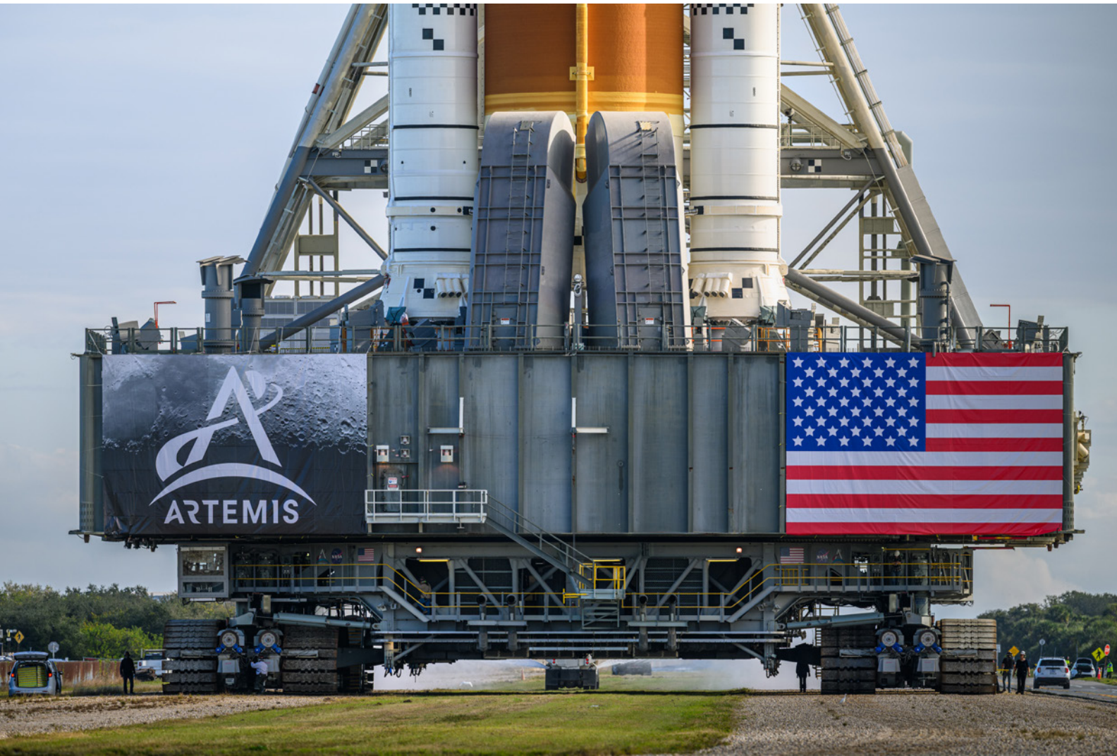
The rollout of the NASA Artemis II rocket at the Kennedy Space Center in Cape Canaveral, Florida on Saturday, January 17, 2026. The crew is spraying water onto the crushed rock track (shown in the bottom of the image) that the crawler is driving over and the maximum speed of the crawler is a slow 0.83 miles per hour (1.3 kph). I will have a full article on my experience photographing the Artemis II Launch in the Summer 2026 issue of the Newsletter.
