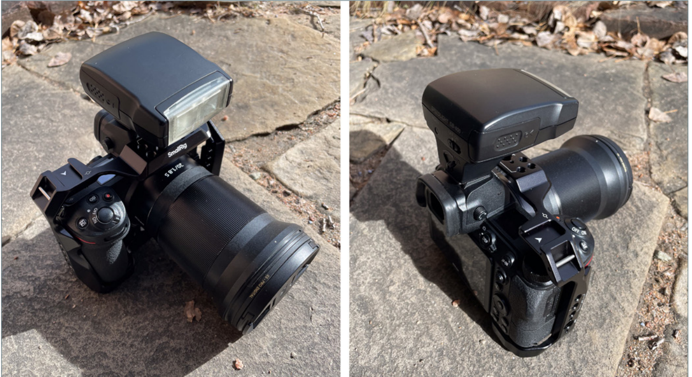
Above is my Nikon Z6 prepped for mounting onto Mike Brewer's helmet for the air-to-air images. The camera is shown here with a SmallRig cage. The cage allowed us to mount the Z6 vertically on the helmet so we could get a horizontal image. Before we finalized the setup on Mike's helmet, we removed the cage to lighten the camera and I also wrapped the flash and camera in a lot of gaffer's tape just to make sure the flash—which was mostly plastic—wouldn't break off in flight.
