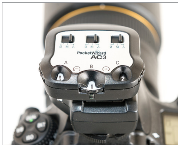
The PocketWizard MiniTT1 Transmitter (top left), seen here atop a Nikon D800, is the main controller for the FlexTT5 Transceiver as shown with a Nikon SB-900 Speedlight mounted on top of it (right). The AC3 ZoneController (bottom left) sits on top of the MiniTT1 and has three rotating dials that let us change the power output on the Speedlight or strobe wirelessly. Together this system allows for reliable triggering of any number of flashes.
